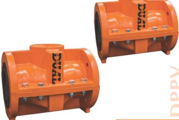
The valve closes by means of air or hydraulic pressure placed on the sleeve, through the top of the valve housing. The valve body acts as a built-in actuator.
