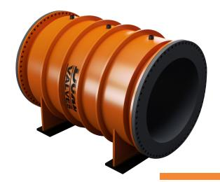
The valve closes by means of air or hydraulic pressure placed on the sleeve, through the top of the valve housing. The valve body acts as a built-in actuator.
