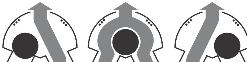
Flow From Right Pump Flow From Both Pumps Flow From Left Pump
